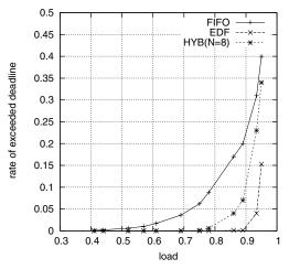
Figure 4. Comparison EDF, FIFO and HYB (N=8)
