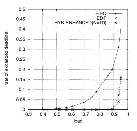
**Figure 7.** Comparison EDF, FIFO and HYB-ENHANCED (N=10)
