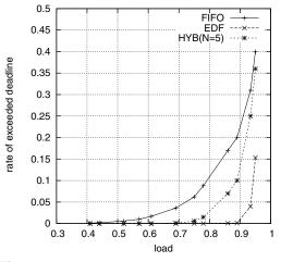
Figure 2. Comparison EDF, FIFO and HYB (N=5)
